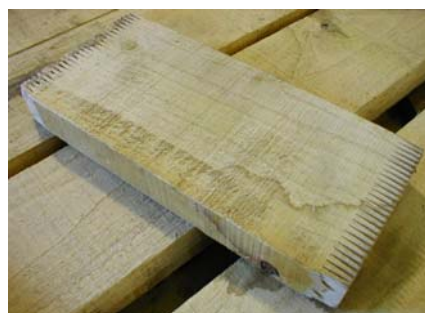
Lengths as short as 125mm can be fingerjointed into 6 metre lengths
